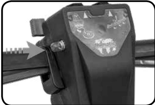
Press re-set switch to reset machine after trip out.
