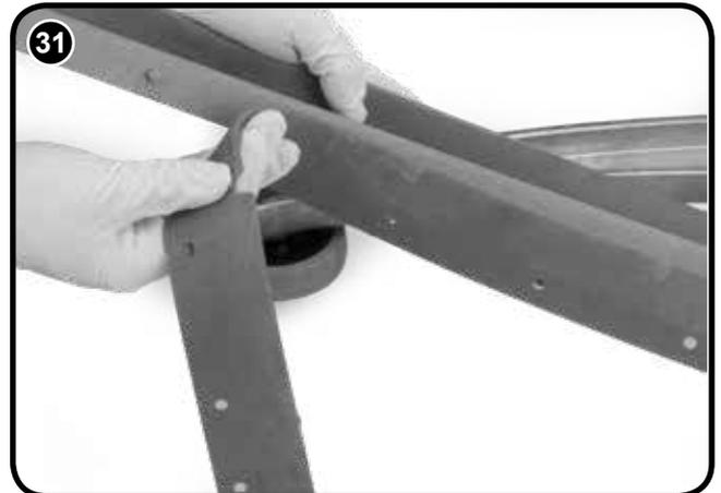
Periodically the floor-tool blades should be examined and checked for wear and damage.
