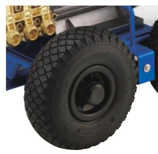
The big, wide pneumatic wheels make the MC 8P very stable and also easy to move around on uneven ground. The parking brake ensures that the machine can be used in all security.
