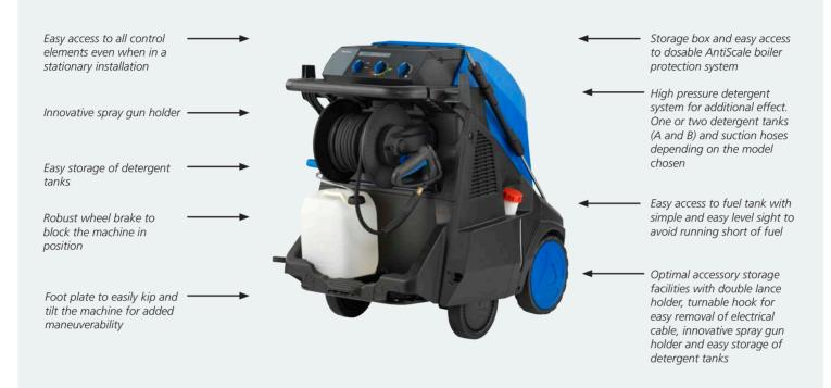
Optimal manoeuvrability and ease of transport – the new design with improved centre of gravity, layout of parts and 4 large wheel design base improves manoeuvrability over all types of surface.
