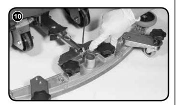
The lifting strap is held by a detent pin (Fig.10).
