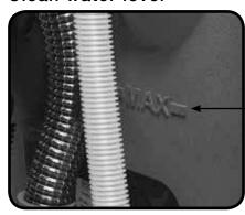
The water level in the clean-water tank can be seen using the clean-water clear dump hose fitted to the rear of the machine.
