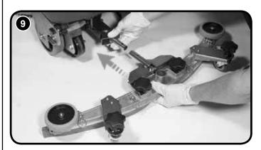
Fit the floor-tool and retain using the detent pin (Fig.9).
