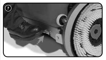
To tip the deck into the down position (Operating mode). Press in the brush deck locking pin (Fig.7) and rotate the brush deck (Fig.8).
