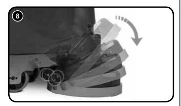
To change to brush deck up position, (Transit mode) simply lift the deck and the sprung loaded locking pin will activate to hold the deck up.
