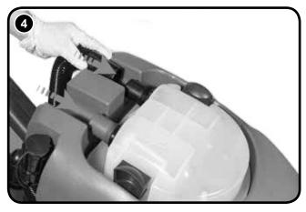
Fit both vacuum and floor-tool hose to the separator (Fig.4).
