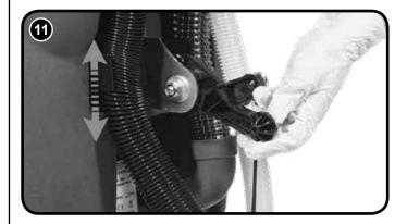
Raise the floor-tool for transit or lower for cleaning operation using the lifting handle fitted to the back of the machine (Fig.11).
