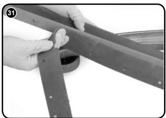
Periodically the floor-tool blades should be examined and checked for wear and damage. The blade removal is easy. Simply start by removing the four retaining pins (see Fig.29), turn the floor-tool over and separate the blade carrier from the body (see Fig.30). Peel away the blades from their locating lugs (see Fig.31) and examine or renew as required. Replacement is a reversal of the removal process.
