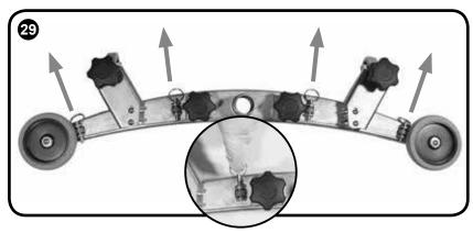
To clean the floor-tool, remove securing-pin and disconnect the lifting strap and remove the floor-tool securing pin pull-free the floor-tool from the rear of the machine. Rinse the floor-tool assembly with clean water and refit.
