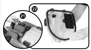
Remove the two hoses to disconnect the separator from the machine (Fig.21).
